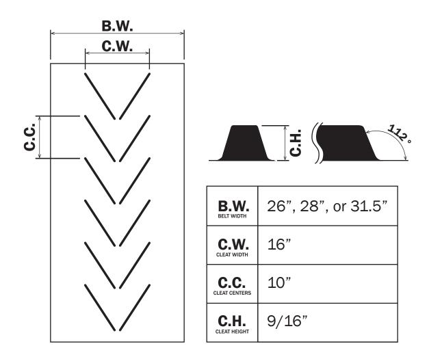
This Integrally Molded Cleat Pattern is used extensively on mobile screening equipment. Mulhern Belting is now stocking this specification on a 2-ply 220 3/16 x 1/16 base belt for immediate shipment. Call for a quote today!
