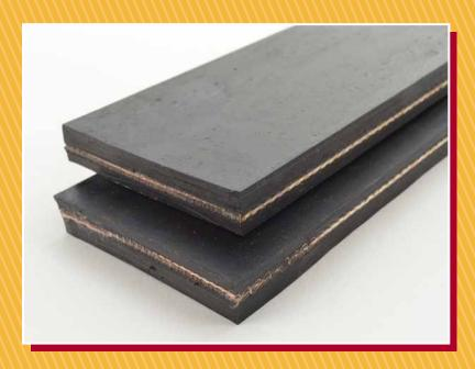
Color: Black Nominal OAG: 0.500" +/- .030 Plies: 1 Fabric: Polyester/Nylon Minimum Pulley Diameter: 20" Top Surface: 1/4" SBR Bottom Surface: 1/8" SBR Compound: SBR Work Tension: 440 lbs. PIW Elongation: less than 4% Weight P.I.W. / Ft: 0.269 Working Temperature: -20F to 250F Joining Method: R5/R6 Lacing
