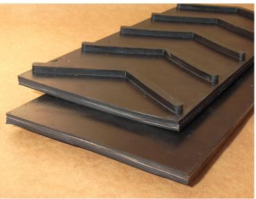
**Features:** 5-8531 features 1/4" high, 6" wide chevron profiles in a staggered pattern. The OAG includes the profile. Use Recessed OAG for Lacing Recommendation.
